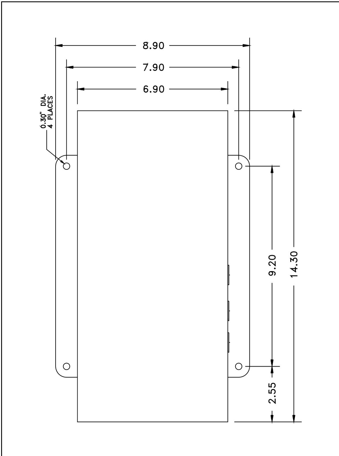
Figure 17. System 1100 Mounting Dimensions.
