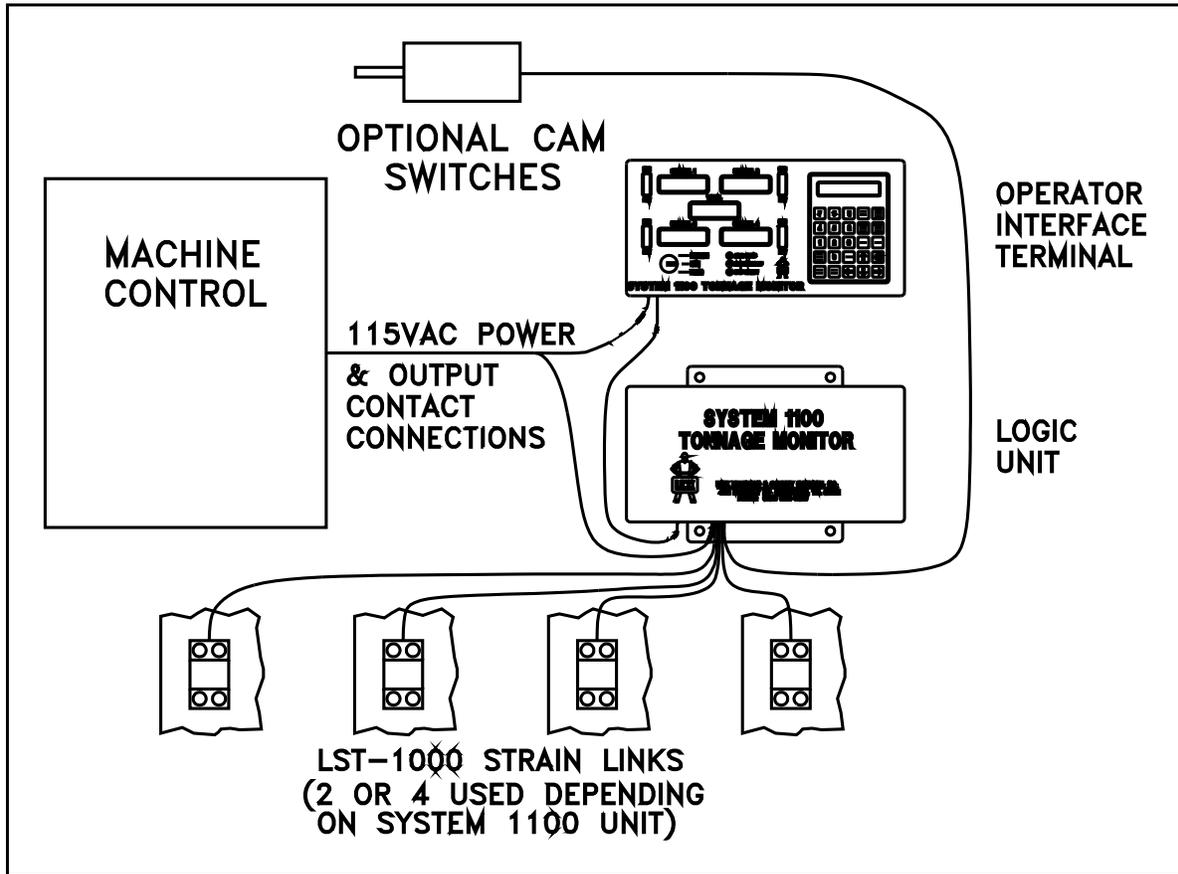
Figure 2. System Components for Panel-mount System 1100.
