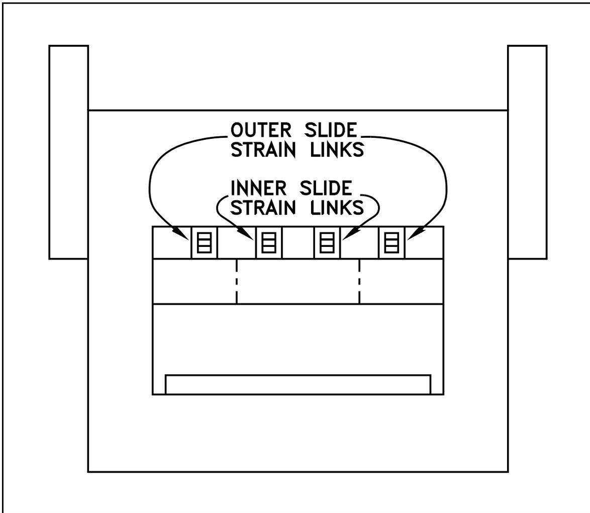
Figure 16. Overdriven Double Action Press.
