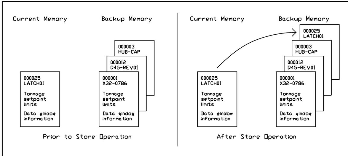
Figure 4. Storing a Setup.
