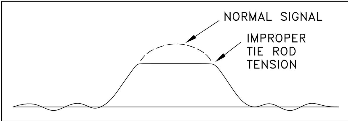
Figure 28. Clipping Due to Improper Tie Rod Tension.
