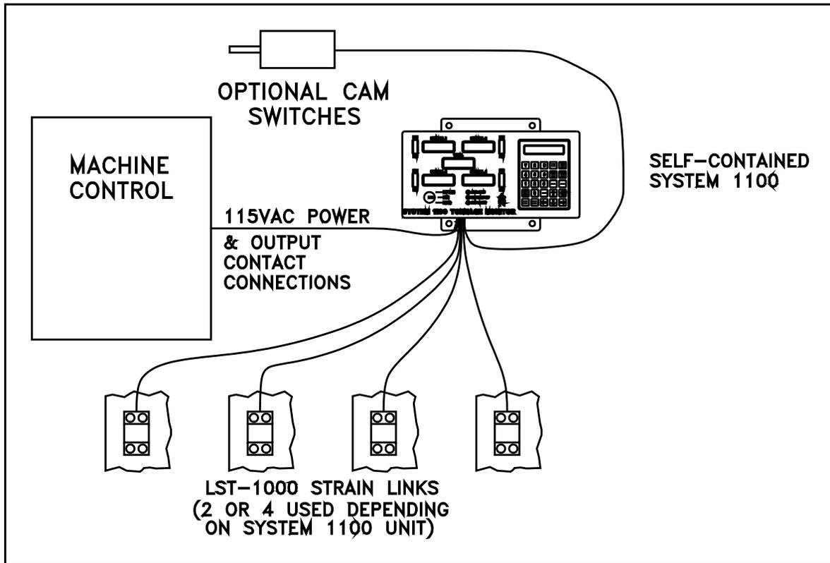
Figure 1. System Components of Self-contained System 1100.
