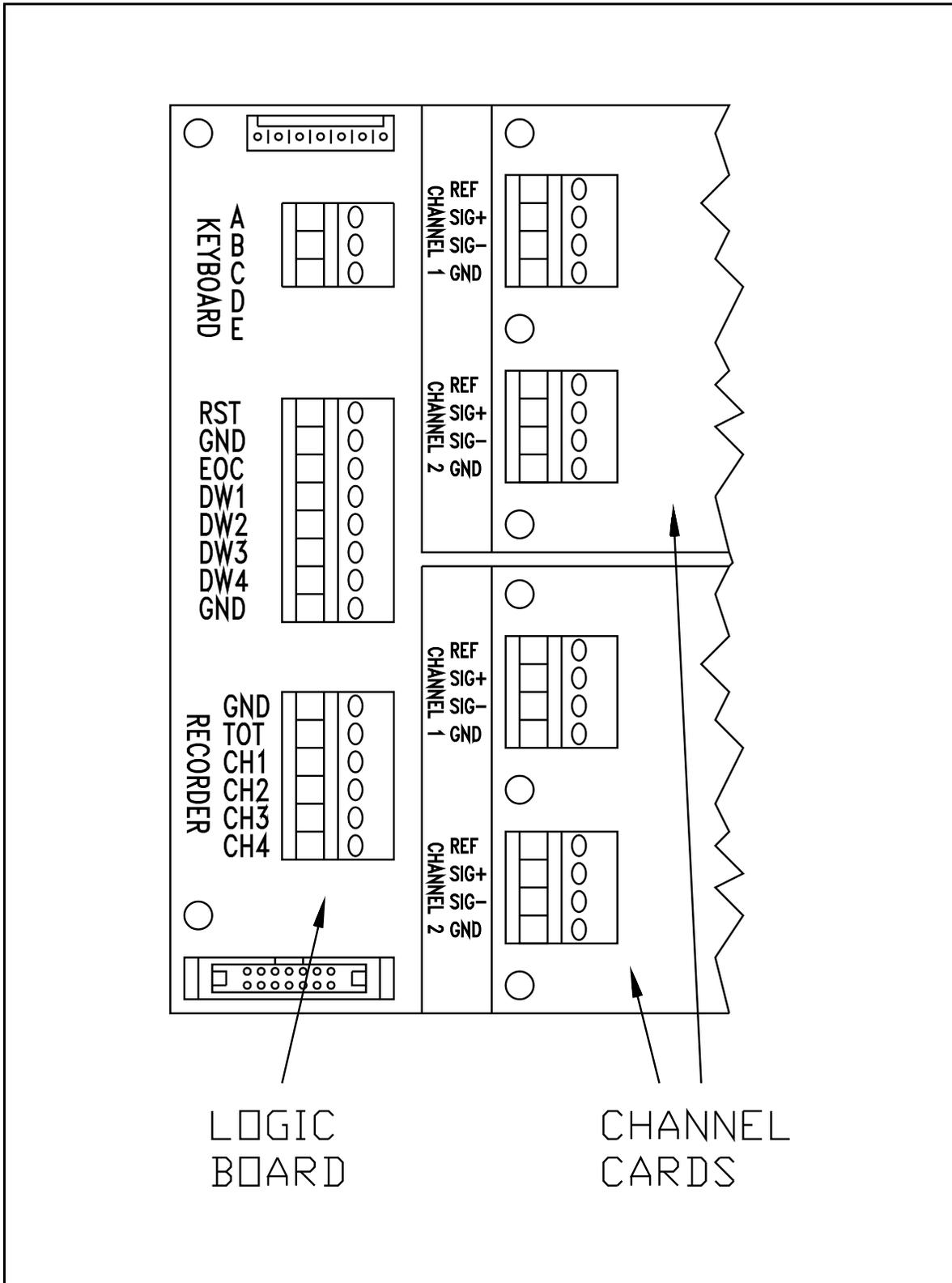
Figure 26. System 1100 Logic Unit Electrical Connections.
