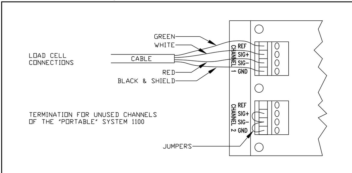
Figure 27. Portable Unit Load Cell & Unused Channel Connection.
