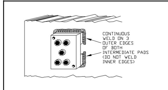
Figure 22. LST-1000 Weld Pads.
