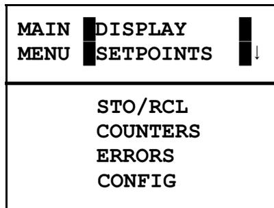
Only two menu options can be shown at one time on the LCD display; the remaining options are accessible by using the up and down arrow keys. If options are available either above or below the currently displayed menu options, then up or down arrows will appear on the right side of the menu indicating so.
